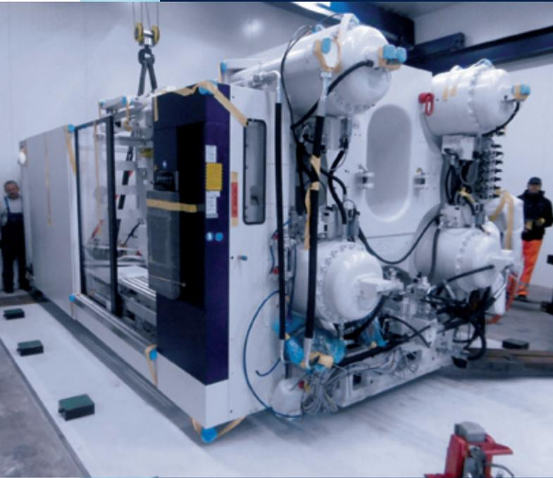
with the clamping unit and injection unit separated - unloaded and transported to its working area by means of a truck-mounted crane, indoor crane and lift truck. There, the two components were fitted together by technicians. With this addition, KH Foliotec is well equipped for the trend to increasingly larger sized parts and tools.
